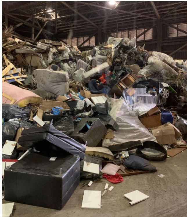
Figure 42: The tipping floor at the WtE facility
