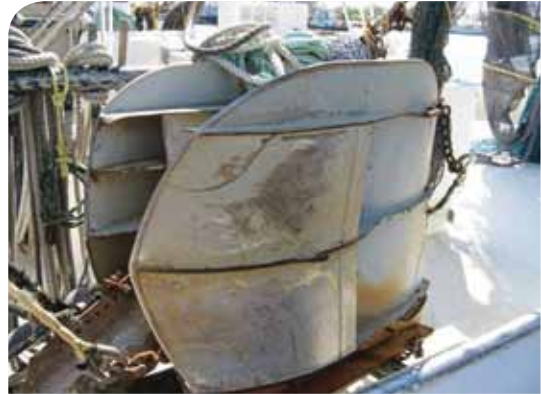
Figure 6.10. Shrimp fishermen using steel cambered trawl doors combined with hydrodynamic nets experience significant fuel savings, less wear on engines and lower maintenance costs.
