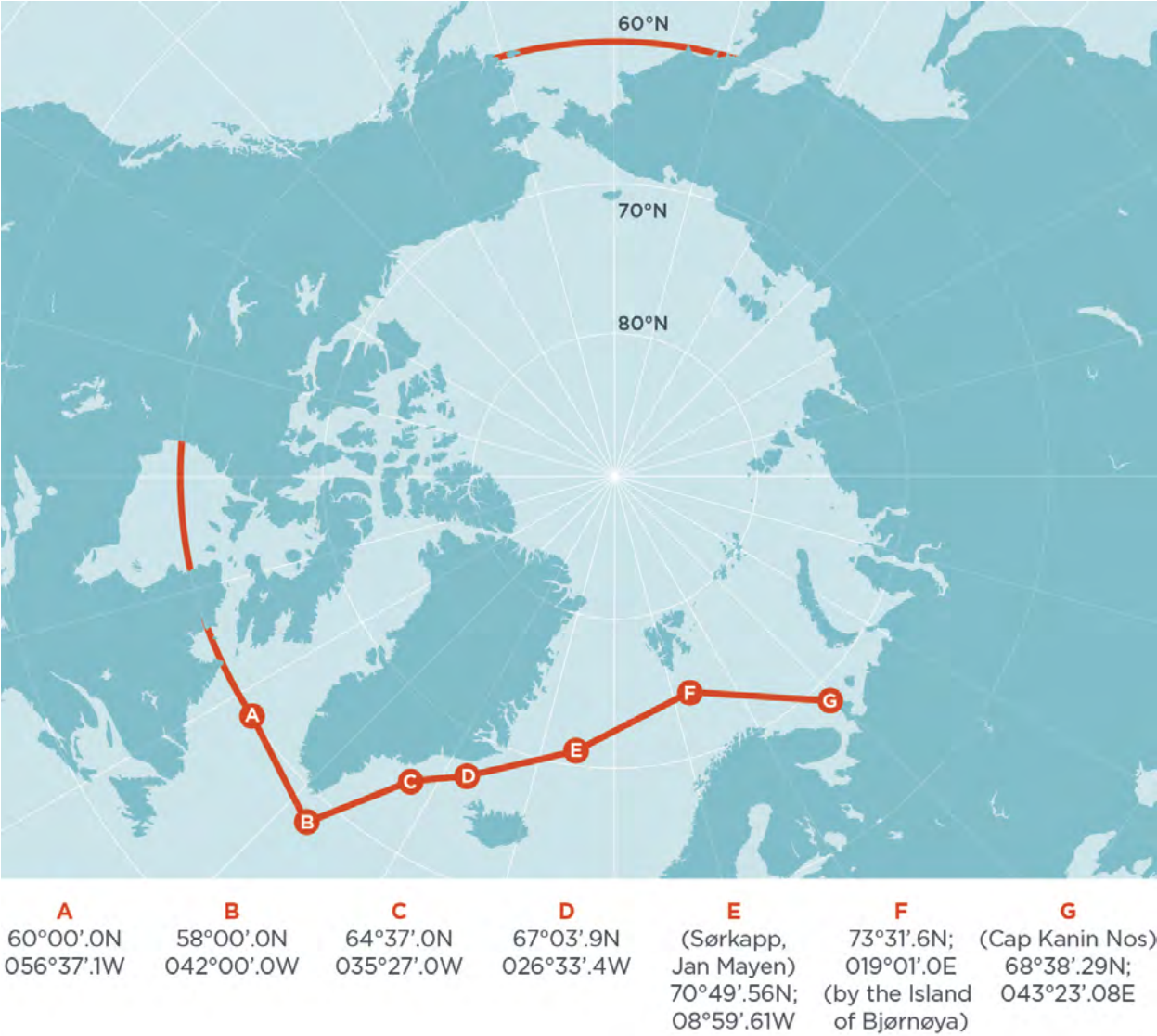
Figure 1: IMO Arctic Polar Code boundaries (i.e., all waters north of the red lines). From [9], adapted from [10].
