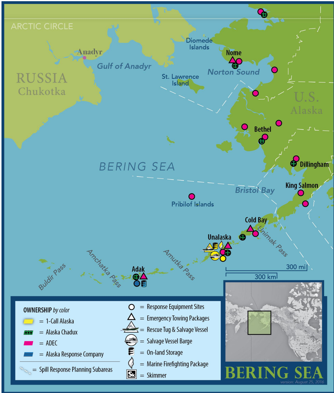
Figure 8-5 Response resources located around the U.S. Bering Sea. Assets are primarily designed for response to small spills in the nearshore, shoreline, or inland areas. Additional assets would be mobilized from other parts of Alaska and the Lower 48 as needed and weather permitting. Map developed based on information from APCs shown in table above. Information is subject to change.
